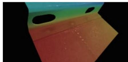
steel plate workpiece point cloud
