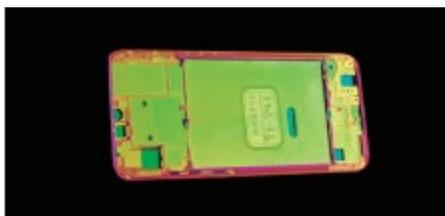
Cell phone center frame hole detection point cloud
